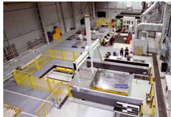
LK V-R twin-rail mounted bridge style CMM
